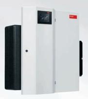
TransTherm giro plus (10, 20, 40) Compact heat transfer station with integrated fresh water module and heating valves for refurbishments and new buildings. Heat outputs: 10–91 kW
