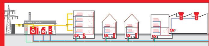
Heating network with Hoyal components; power station with PowerBloc combined heat and power plant (1). UltraGas® heat generator (2) and buffer storage tank (3), TransTherm heat transfer stations (4), TransShare heating distributor (5) and calorifiers (6) – all connected by the TopTronic system controlled
