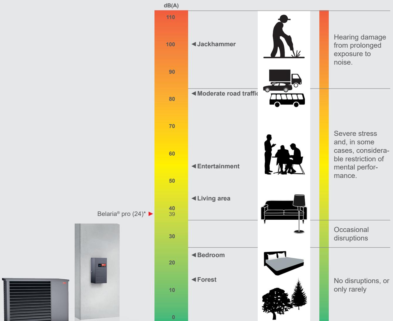
\* at a distance of 5 m if the outdoor unit is positioned against a wall. These values are reduced by 3 dB if the outdoor unit is free-standing. With installation in a corner, the sound pressure level increases by 3 dB. The sound values apply with a clean evaporator. These values are temporarily exceeded shortly before defrosting.
