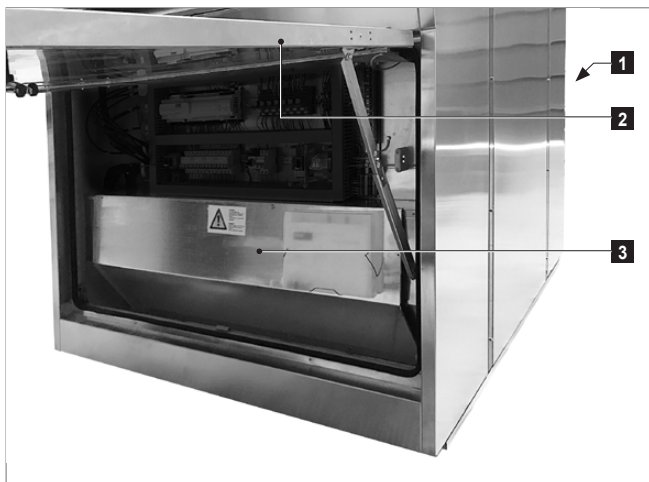
Fig. 15: The fan protecting plate is temporarily attached with 4 screws during delivery.
