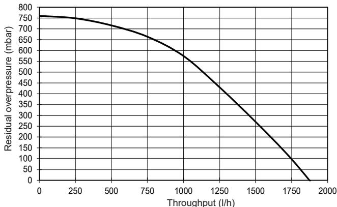
**Residual overpressures of heating pump**
