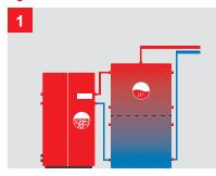
Hybrid system with renewable energy. Use of renewable energy (geothermal heat pump). Base load is covered by the heat
