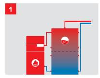
System solution with wood pellet boiler. Meets the relevant legal regulations (the "Renewable Energies Heat Act", or EEWärmeG, and the "Model cantonal provisions in the energy sector", or MuKEn); base load is covered by the wood pellet boiler.
