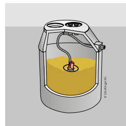
Concrete pellet tank with mole output system
