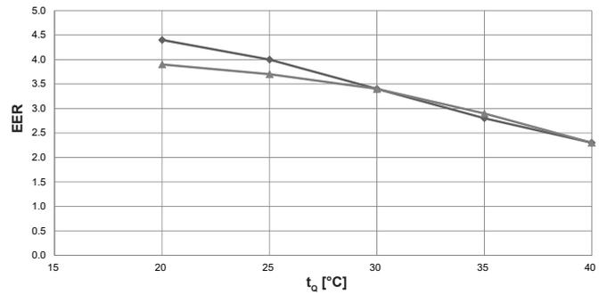
Cooling capacity -  $t_{VL} 18\text{ °C}$
