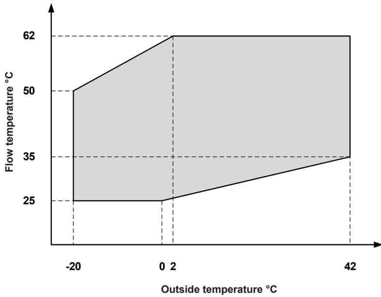
Area of application of the heat pump for heating
