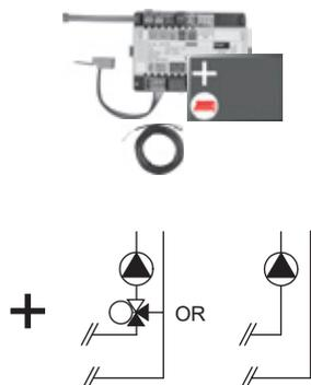
**TopTronic® E module expansion heating circuit TTE-FE HK**
