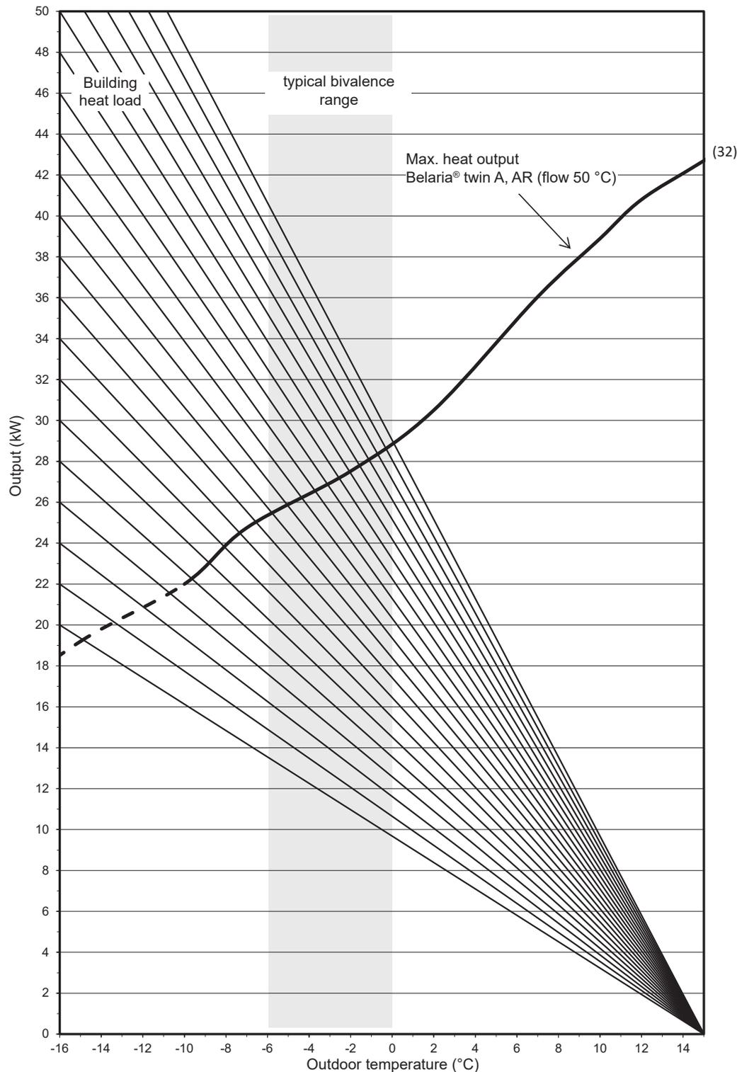
**Dimensions of the Belaria® dual AR air/water heat pump with panel heating**
