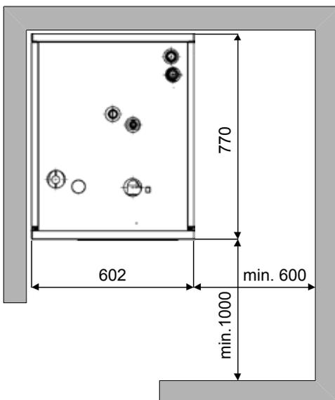
Due to the need for access to the 3-way switching ball valve for heating and domestic hot water, a gap of at least 600 mm must be guaranteed on the right side.
