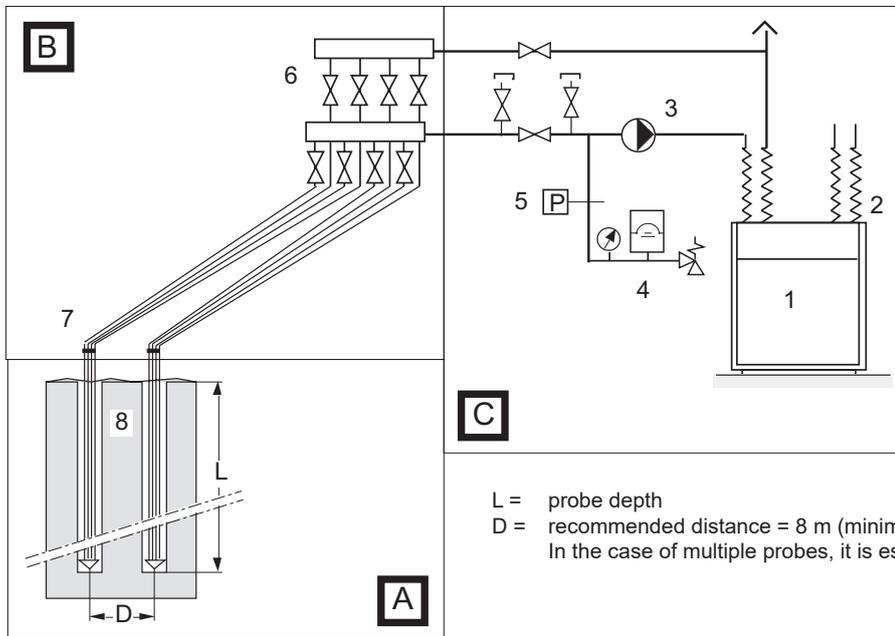
**Field A) Geothermal probes**
