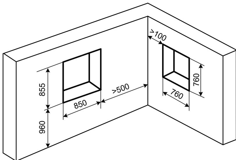
Space requirement “Flex” installation with wall insulation MI, outlet on top via flexible hose
