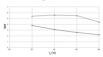
$\begin{array}{ll} t_{_{VL}} &= cooling \ water \ flow \ temperature \ (^{\circ}C) \\ t_{_{O}} &= source \ temperature \ (^{\circ}C) \\ Q_{_{k}} &= cooling \ capacity \ (kW), \ measured \ in \ accordance \ with \ standard \ EN \ 14511 \\ EER &= Energy \ Efficiency \ Ratio \ for \ the \ overall \ unit \ in \ accordance \ with \ standard \ EN \ 14511 \end{array}$
