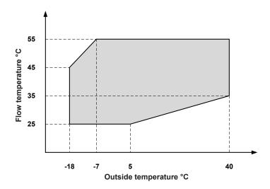
Area of application of the heat pump for domestic hot water
