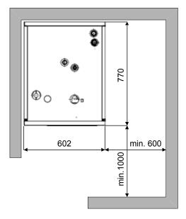
Due to the need for access to the 3-way switching ball valve for heating and domestic hot water, a gap of at least 600 mm must be guaranteed on the right side.
