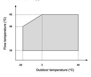
Area of application of the heat pump for heating/domestic hot water
