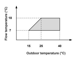
Area of application of the heat pump for heating/domestic hot water
