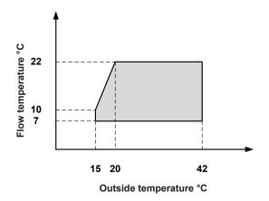
Area of application of the heat pump for cooling
