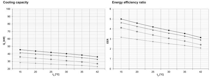
= source temperature (°C) = cooling capacity at full load (kW), measured in accordance with standard EN 14511
