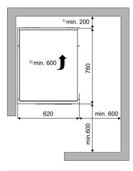
1) A gap of at least 200 mm must be guaranteed at the rear for the refrigerant as well as electrical connection.
