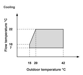
Area of application of the heat pump for cooling
