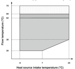
Area of application of the heat pump for heating (UltraSource® T comfort C and compact C)
