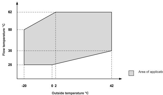
Area of application of the heat pump for heating
