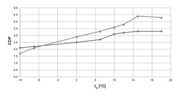
$\begin{array}{ll} t_{_{VL}} &= \text{heating flow temperature (°C)} \\ t_{_{Q}} &= \text{source temperature (°C)} \\ Q_{_{h}} &= \text{heat output (kW), measured in accordance with standard EN 14511} \\ \text{COP} &= \text{Coefficient of Performance for the overall unit in accordance with standard EN 14511} \end{array}$
