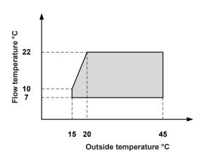
Area of application of the heat pump for cooling
