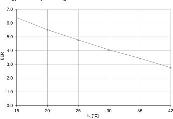
t<sub>vi</sub> = cooling water flow temperature (°C)
