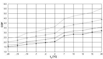
$egin{array}{ll} t_{_{O}} &= source\ temperature\ (^{\circ}C) \\ Q_{_{h}} &= heat\ output\ at\ full\ load\ (kW),\ measured\ in\ accordance\ with\ standard\ EN\ 14511\ COP = Coefficient\ of\ Performance\ in\ accordance\ with\ standard\ EN\ 14511 \\ \end{array}$
