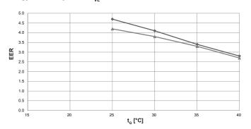
$\begin{array}{ll} t_{_{VL}} &= cooling \ water \ flow \ temperature \ (^{\circ}C) \\ t_{_{O}} &= source \ temperature \ (^{\circ}C) \\ Q_{_{k}} &= cooling \ capacity \ (kW), \ measured \ in \ accordance \ with \ standard \ EN \ 14511 \\ EER &= Energy \ Efficiency \ Ratio \ for \ the \ overall \ unit \ in \ accordance \ with \ standard \ EN \ 14511 \end{array}$
