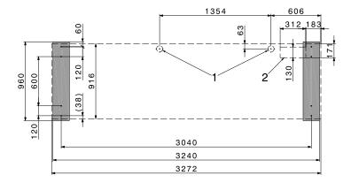
The concrete base must have a level surface the size of the Belaria® dual AR (60). The base should have chamfered edges.
