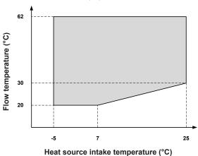
Area of application of the heat pump for heating (UltraSource® T comfort C and compact C)
