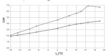
Heat output -  $t_{_{VL}}$  45 °C
