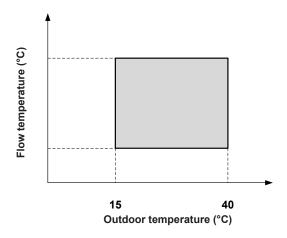
Area of application of the heat pump for cooling (UltraSource® B comfort C and compact C)
