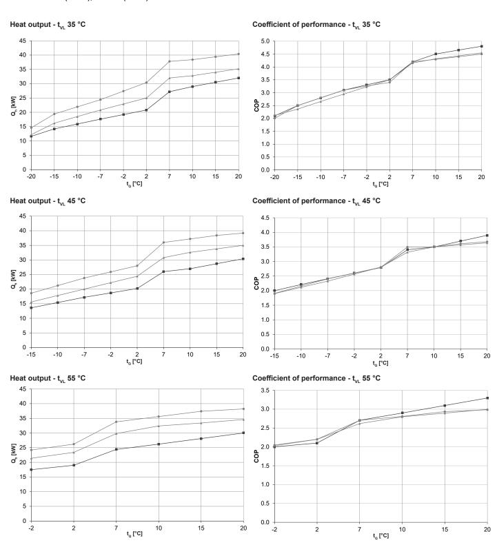
t<sub>vL</sub> = heating flow temperature (°C)
