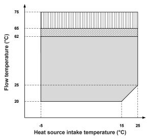
Area of application of the heat pump for heating (UltraSource® T comfort C and compact C)
