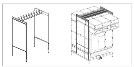
Fig. 11: Lifting beam for unloading the unit
