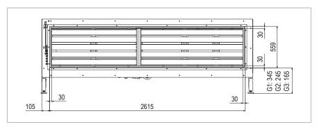
Fig. 14: Dimensions of the fresh air box (in mm)
