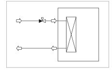
Fig. 23: Connection of the cooling coil
