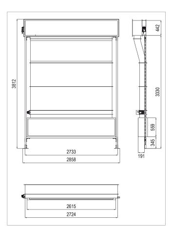
Fig. 17: CPS dimensions (in mm)
