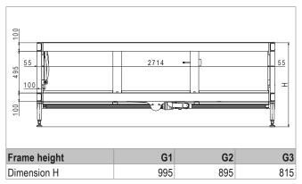
Fig. 21: Dimensional drawing for supply air duct (dimensions in mm)
