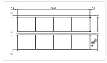
Fig. 20: Dimensional drawing for extract air duct (dimensions in mm) (inspection opening for filter exchange)
