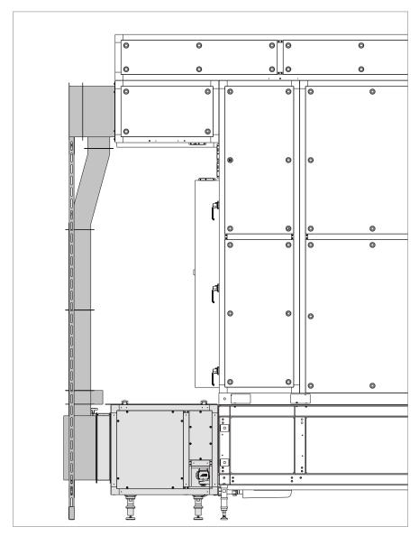
Fig. 7: ServeCool unit with fresh air box and condensation prevention system
