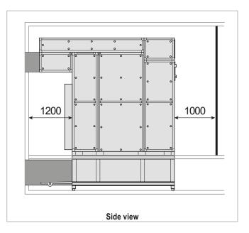
Fig. 9: Space requirements for maintenance and servicing (minimum clearances in mm)
