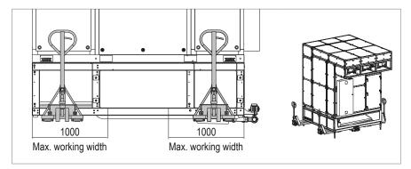
Fig. 12: Positioning the lifting truck
