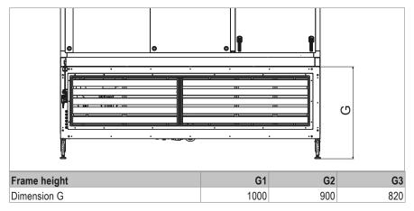
Fig. 5: Dimensional drawing frame height (dimensions in mm)
