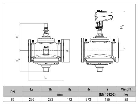
Fig. 6: Cooling valve dimensional drawing
