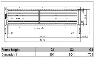
Fig. 22: Dimensional drawing for fresh air duct (dimensions in mm)
