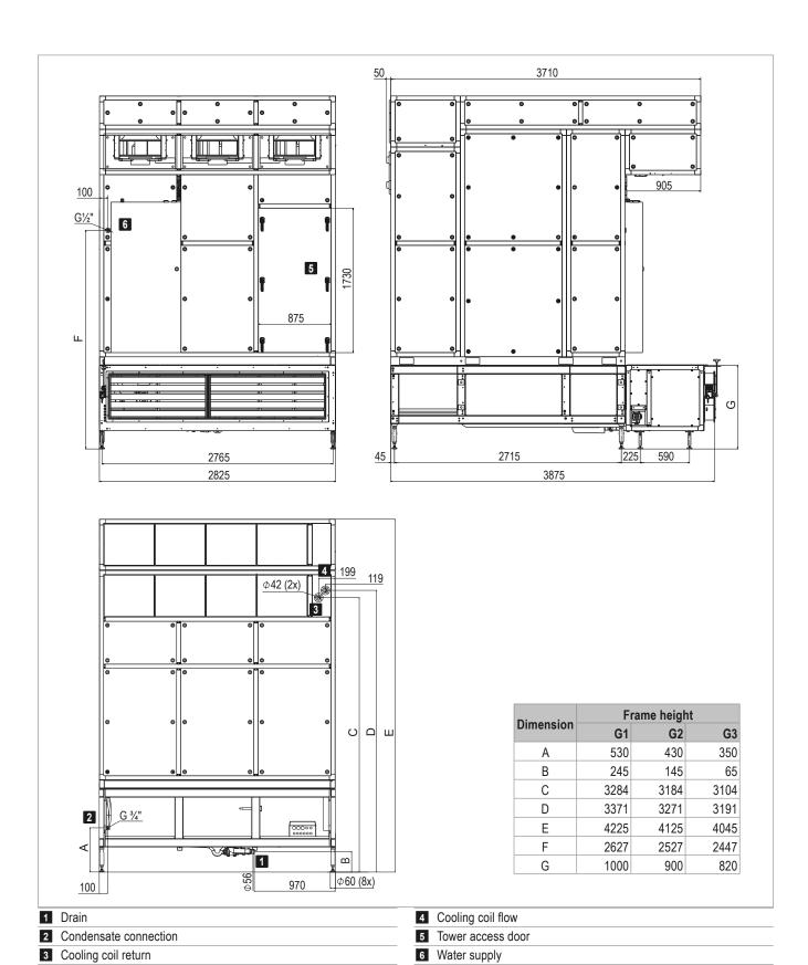
Fig. 4: Dimensional drawing (dimensions in mm)
