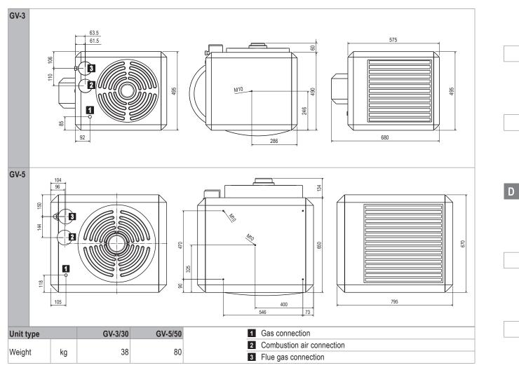
Fig. D2: TopVent® GV dimensions and weights
