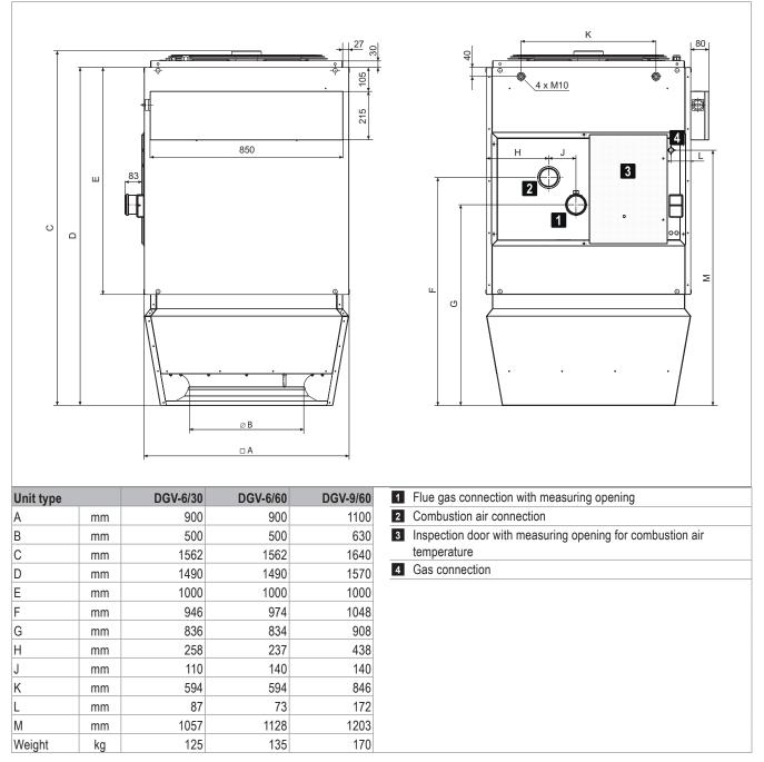
Fig. B3: TopVent® DGV dimensions and weights
