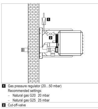
Fig. D5: Gas pressure regulator and cut-off-valve in the gas supply line
