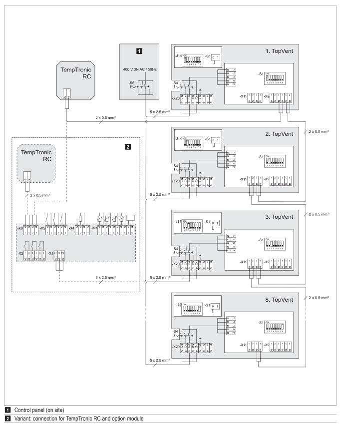
Fig. B5: Connection diagram
