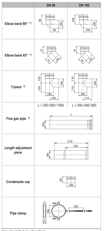
1) Insertion depth of pipe collar = 50 mm
