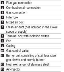
Fig. E1: TopVent® MG structure
