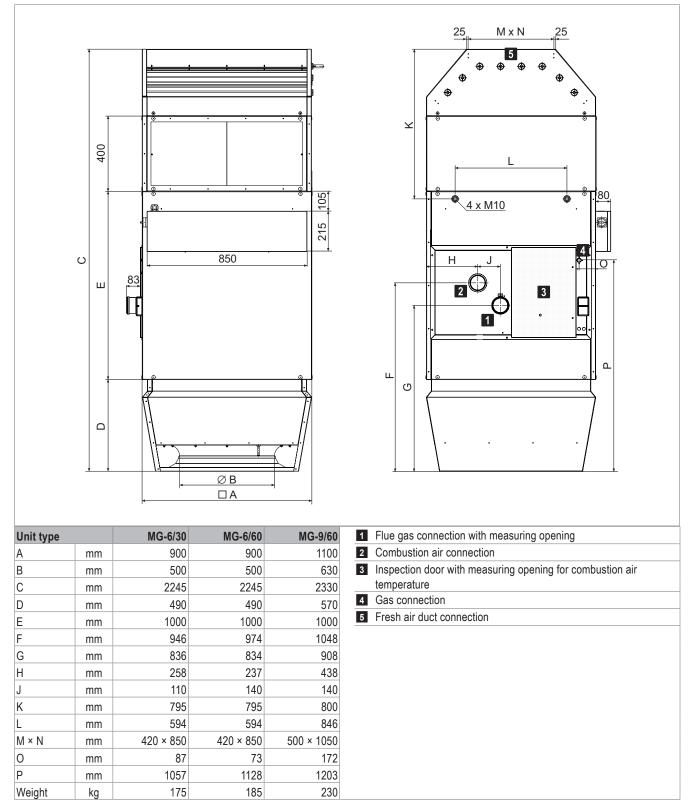
Fig. E3: TopVent® MG dimensions and weights
