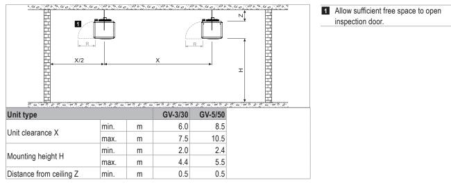
Table D9: TopVent® GV minimum and maximum distances for vertical air flow (ceiling mounting)
