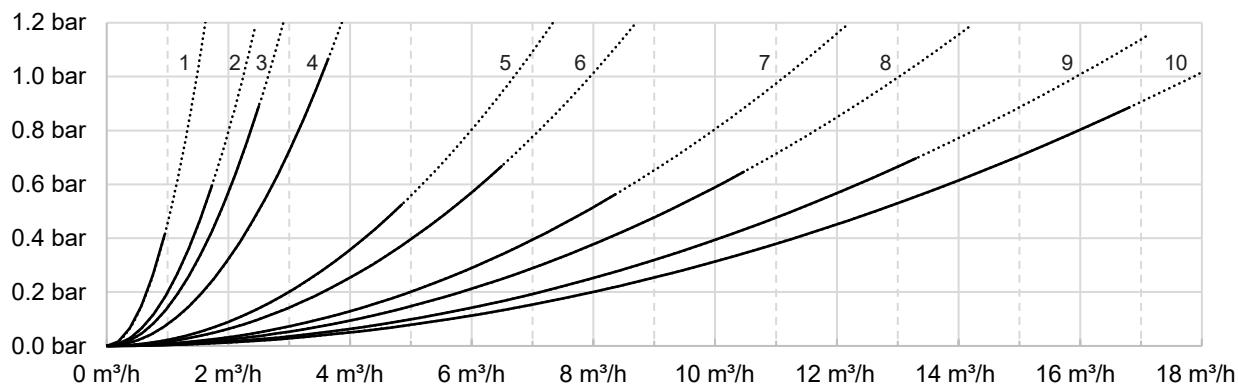
**Residual overpressure / charging circuit flow HT**
