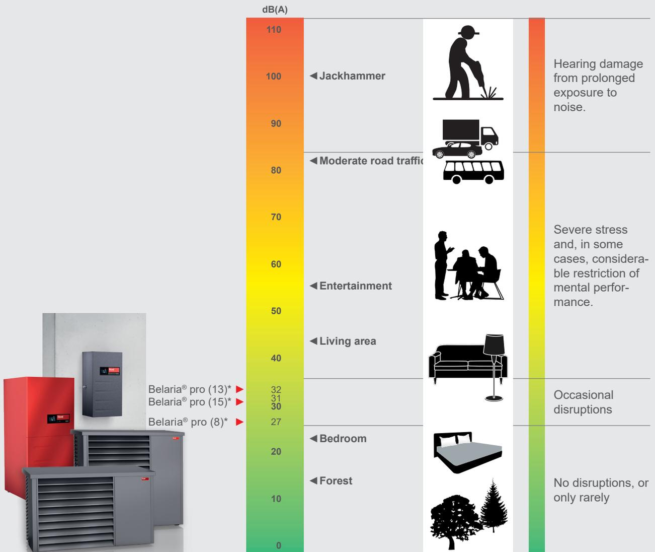
\* at a distance of 5 m if the outdoor unit is positioned against a wall. These values are reduced by 3 dB if the outdoor unit is free-standing. With installation in a corner, the sound pressure level increases by 3 dB. The sound values apply with a clean evaporator. These values are temporarily exceeded shortly before defrosting.
