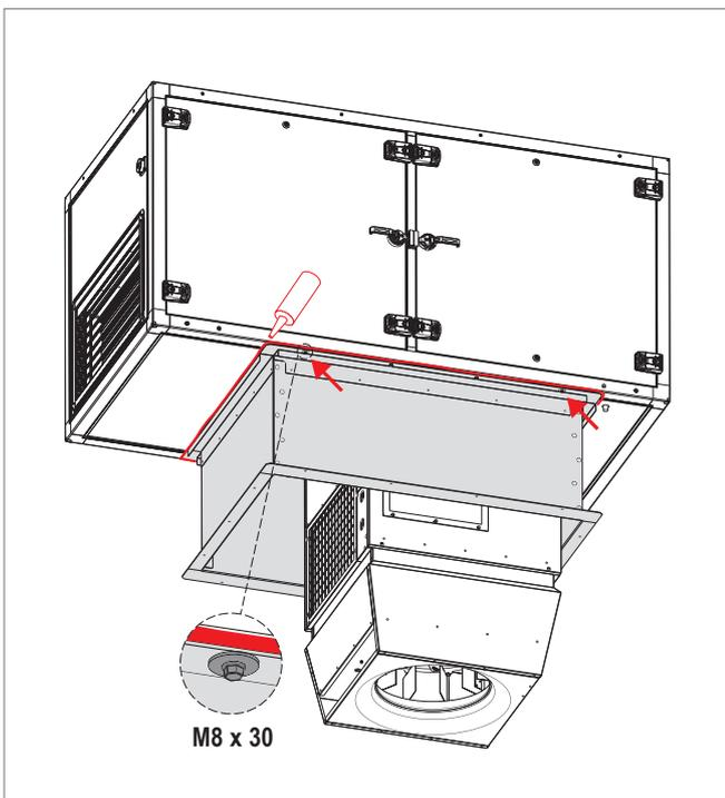
Fig. 32: Screw joint and sealing
