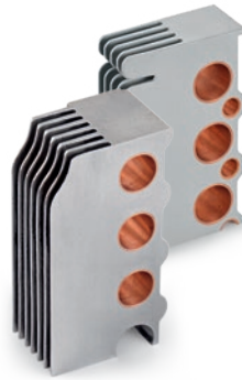
TopGas® heat exchanger: A sophisticated mix of conductive aluminium and corrosion-resistant copper. The TopGas® combi (behind) has an additional copper water channel for water heating.
