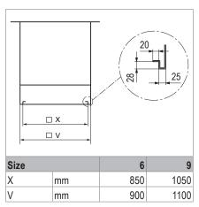
Table 39: Connection dimensions supply air duct (in mm)
