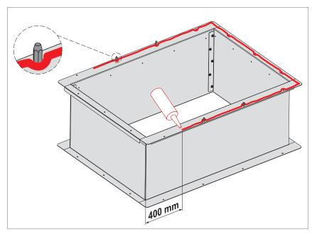
Fig. 28: Applying the sealing compound
