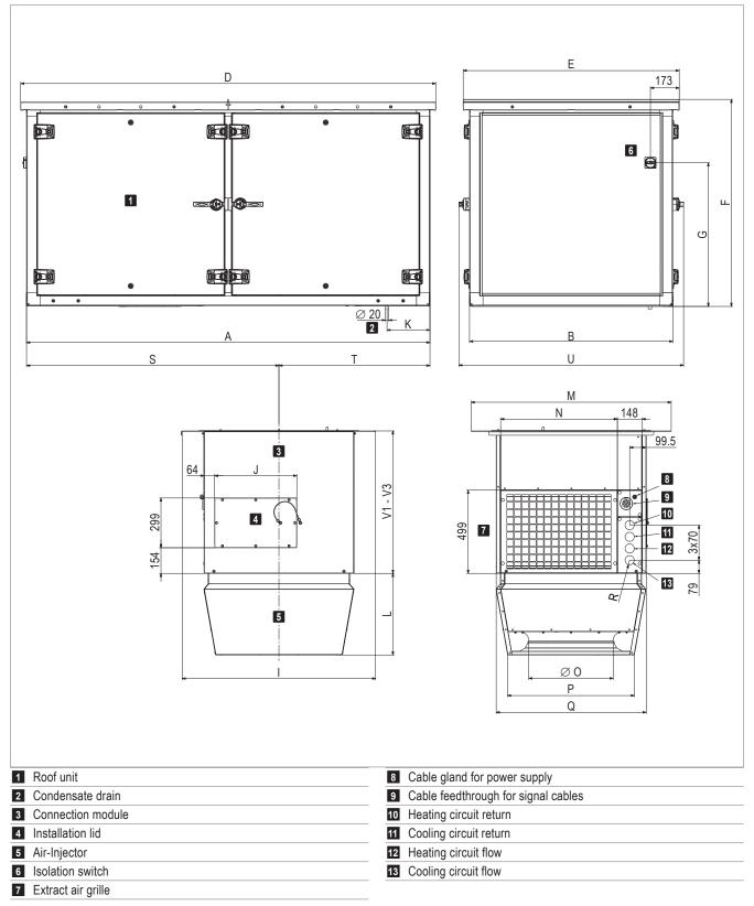
Fig. 16: Dimensional drawing for TopVent® CHC with hydraulic assembly throttling circuit (dimensions in mm)
