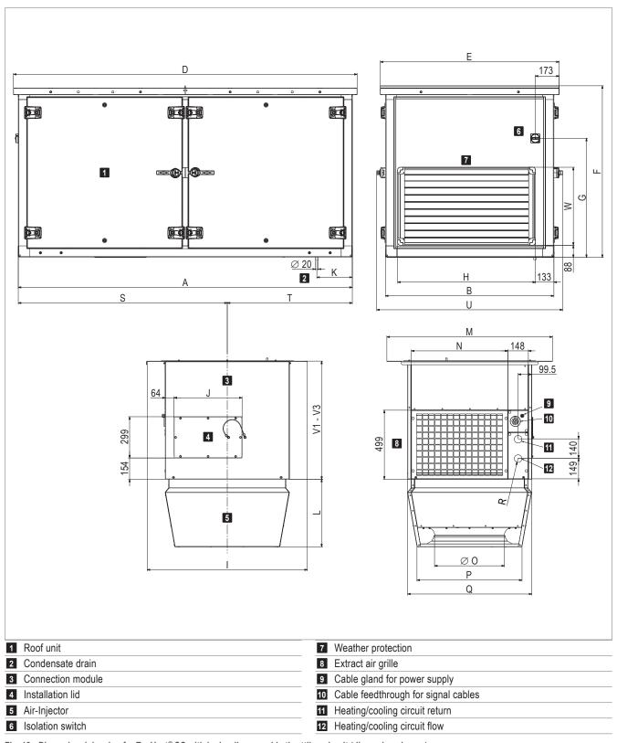
Fig. 18: Dimensional drawing for TopVent® SC with hydraulic assembly throttling circuit (dimensions in mm)
