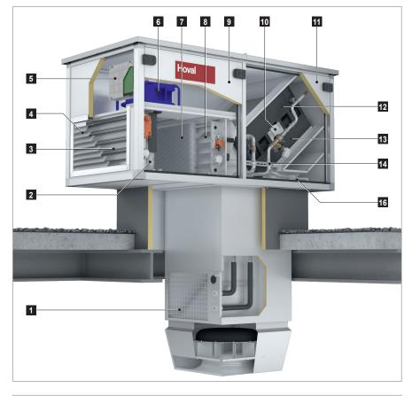
Extract air grille Fresh air filter Fresh air damper Weather protection Unit control box 6 Fan Extract air filter Recirculation damper Fan access door Frost controller 11 Hydraulic connection access door 12 Heating/cooling coil 13 Condensate separator 14 Hydraulic assembly throttling circuit 15 Condensate drain
