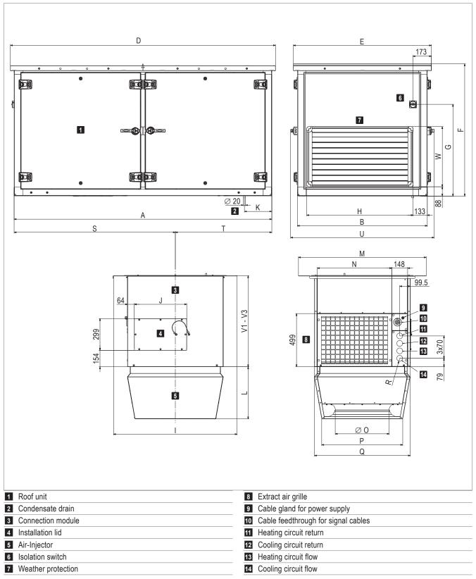
Fig. 19: Dimensional drawing for TopVent® SHC with hydraulic assembly throttling circuit (dimensions in mm)
