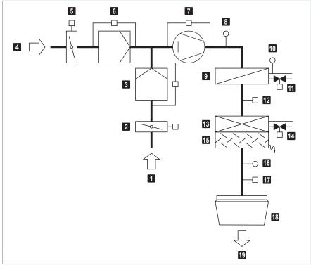
Fig. 12: TopVent® SHC construction
