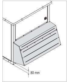
Fig. 34: Protection hood mounted on the roof unit
