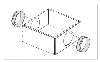
Fig. 35: Mounting the collars
