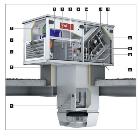
Extract air grille Fresh air filter Fresh air damper Weather protection Unit control box 6 Fan Extract air filter Recirculation damper Fan access door Heating coil Frost controller 12 Hydraulic connection access door 13 Cooling coil Condensate separator 15 Hydraulic assembly throttling circuit 16 Condensate drain
