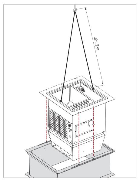
Fig. 29: Hanging the below-roof unit
