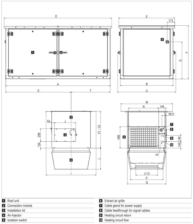
Fig. 14: Dimensional drawing for TopVent® CH with hydraulic assembly throttling circuit (dimensions in mm)
