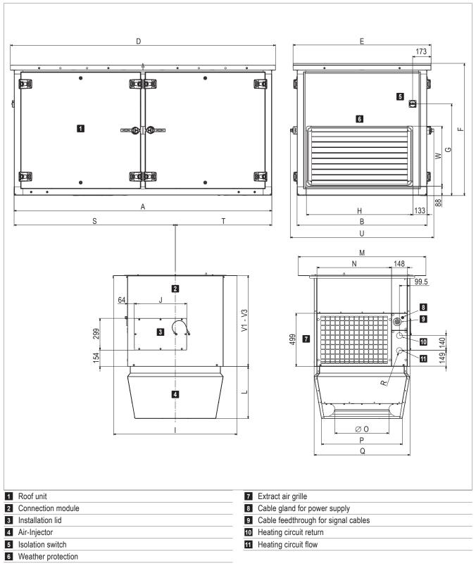
Fig. 17: Dimensional drawing for TopVent® SH with hydraulic assembly throttling circuit (dimensions in mm)
