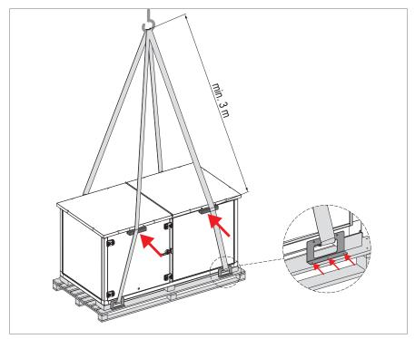
Fig. 30: Lifting the roof unit
