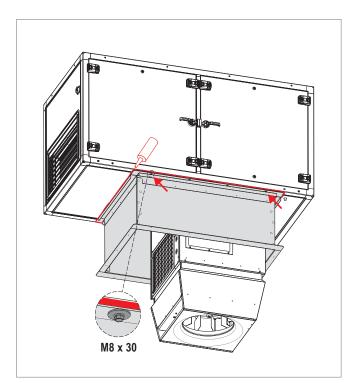
Fig. 32: Screw joint and sealing
