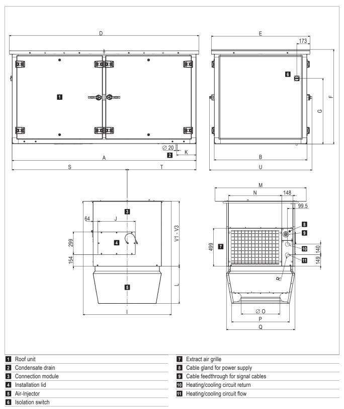
Fig. 15: Dimensional drawing for TopVent® CC with hydraulic assembly throttling circuit (dimensions in mm)
