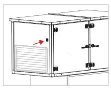
Fig. 44: Position of the isolation switch
