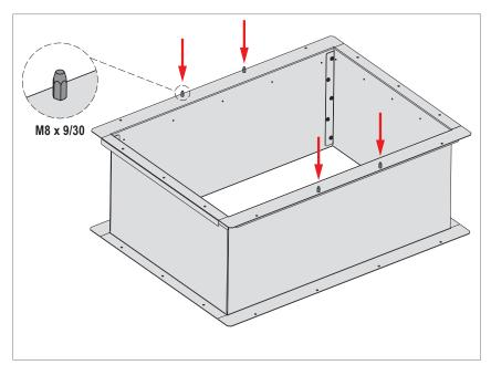
Fig. 27: Adjustment screws in the roof frame
